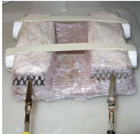
Figure 3: Experimental setup for desalination of single tile
